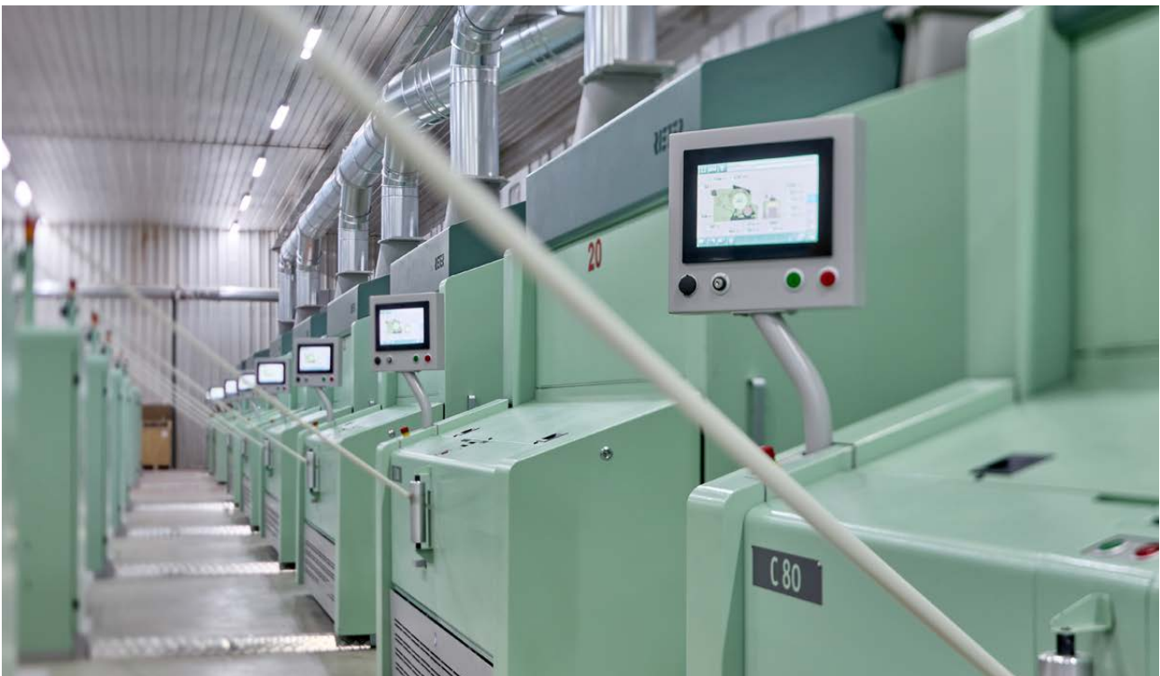
A customer used a blend of 90% recycled cotton for its rotor yarn. The C 80 card is particularly suitable for such applications.
