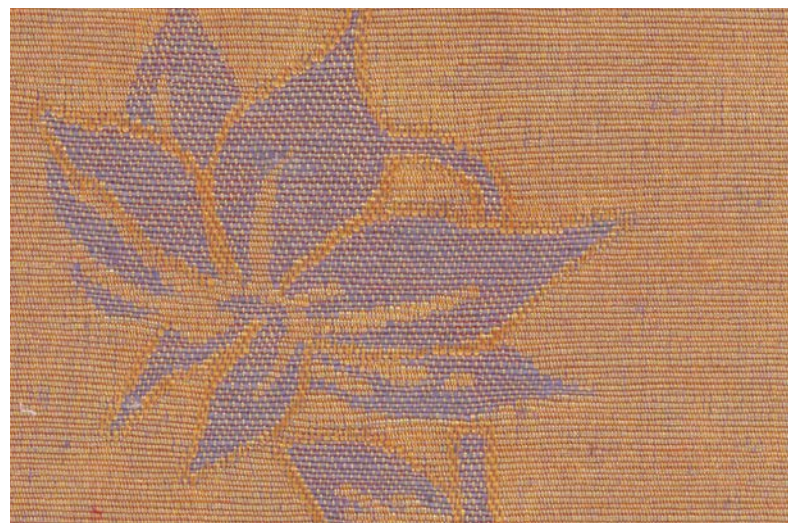
Furnishing fabric warp: 78 dtex polyester filament weft: Nm 9.6 flax yarn, rotor-spun
