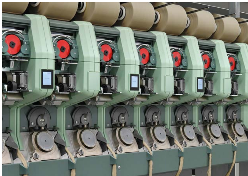
Standard and fancy yarns can be produced economically on a rotor spinning machine.
