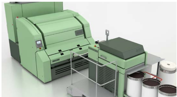
Cards with the RSB-Module 50 deliver the ideal feed sliver for the rotor spinning machine.
