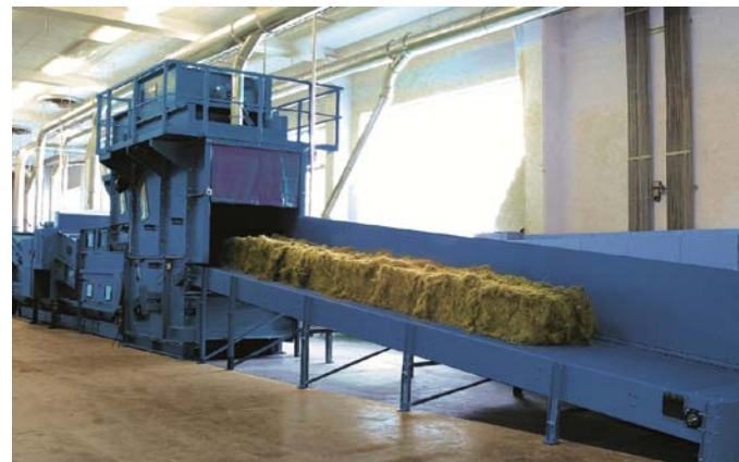
Preparing the flax tow for the spinning mill
