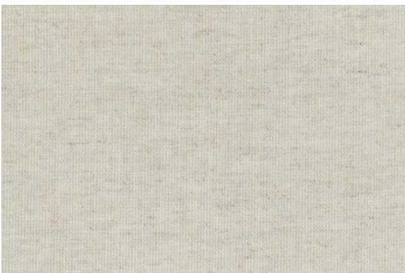
Coating fabric warp: Nm 28/2 cotton yarn, ring-spun weft: Nm 12 flax yarn, rotor-spun
