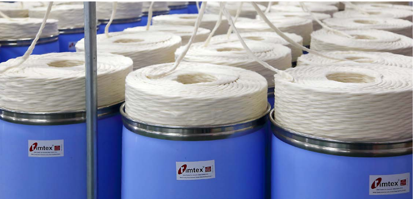
Fig. 1 Rimtex cans guarantee an accurate sliver coiling and a faultless sliver take-off.
