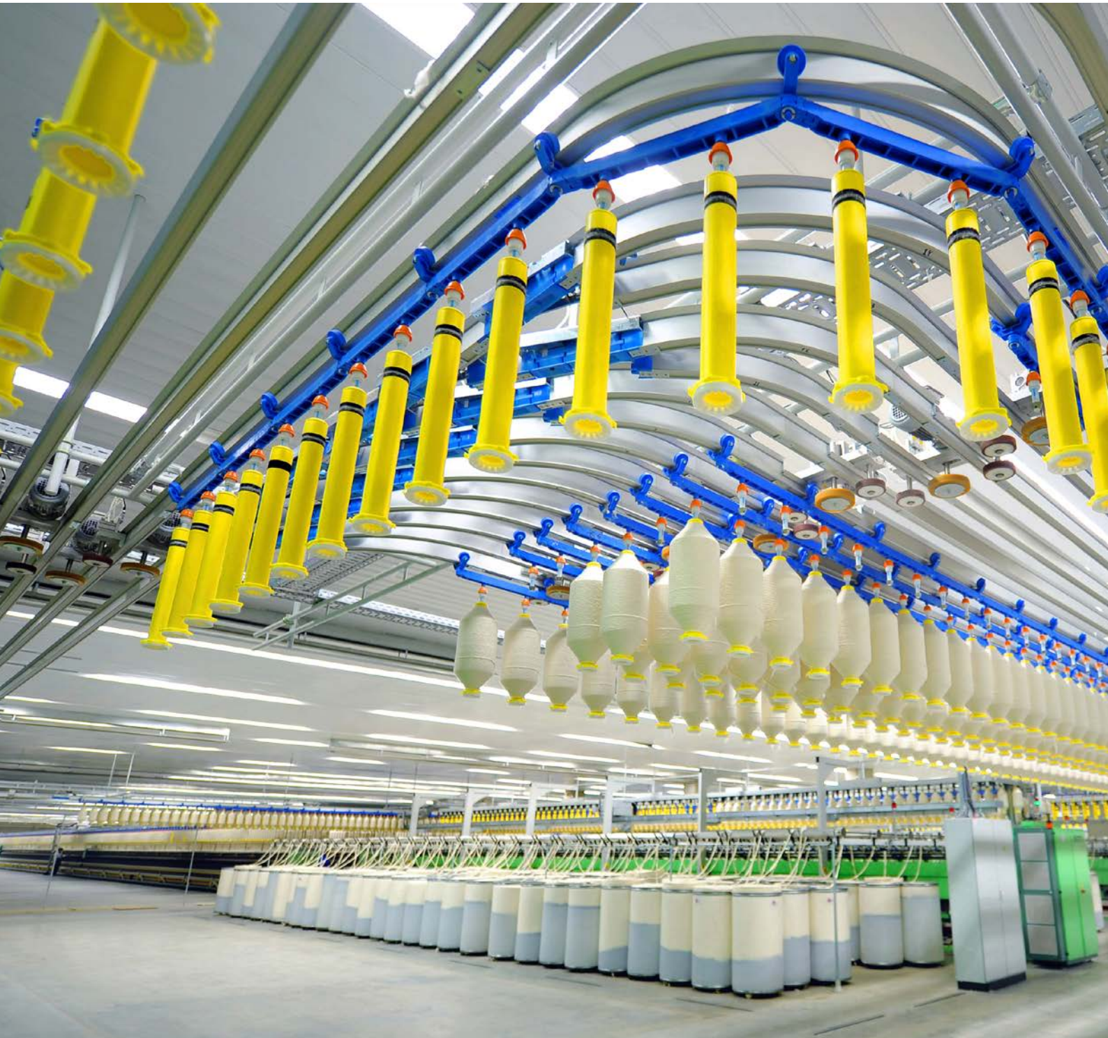
Fig.1 SERVOrail roving bobbin transport system – for efficient and quality-conscious spinning mills.
