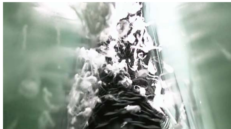
Fig. 3 Gentle, continuous extraction of the microtufts - thanks to patented wobble disc take-off roller.
