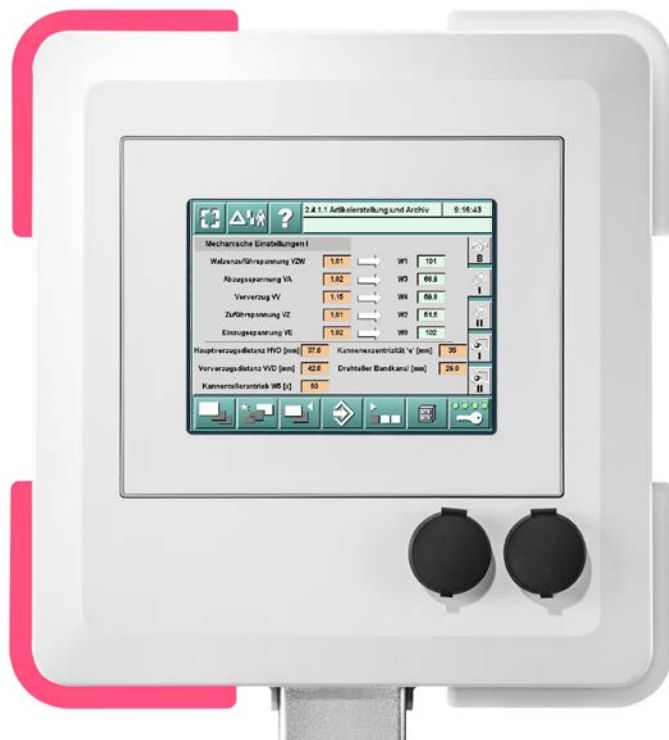
Fig. 8 LEDs visible from afar allow the operators to work efficiently.
