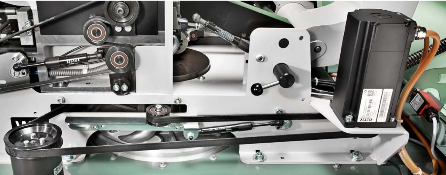
Fig.2 The servomotor for the coiler allows rapid optimization of the speed.
