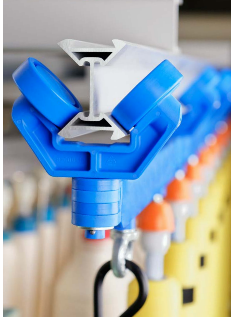
Fig. 4 The tilted sliding surfaces of the aluminium profile prevent soiling and are thus maintenance-free.
