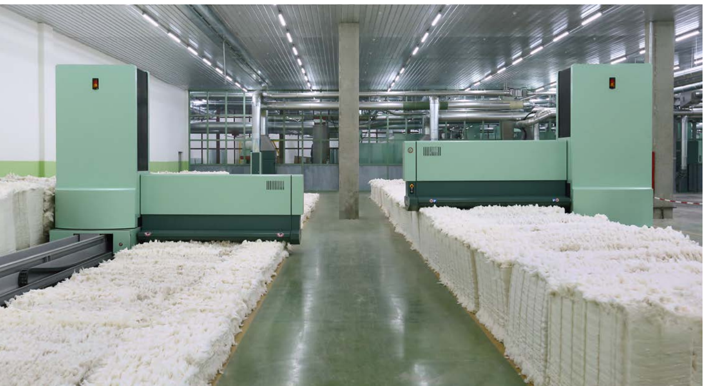
Fig. 1 A 12 UNIfloc – the modern and efficient method of opening bales.
