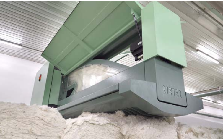
Fig. 2 High production after bale group change thanks to patented bale scanning.
