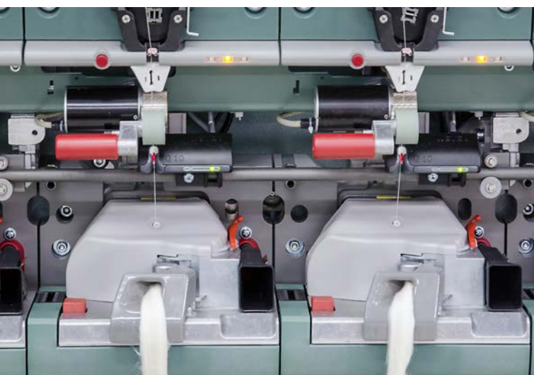
Fig. 2 The modernized S 36 spin box ensures higher yarn strength and fewer imperfections.
