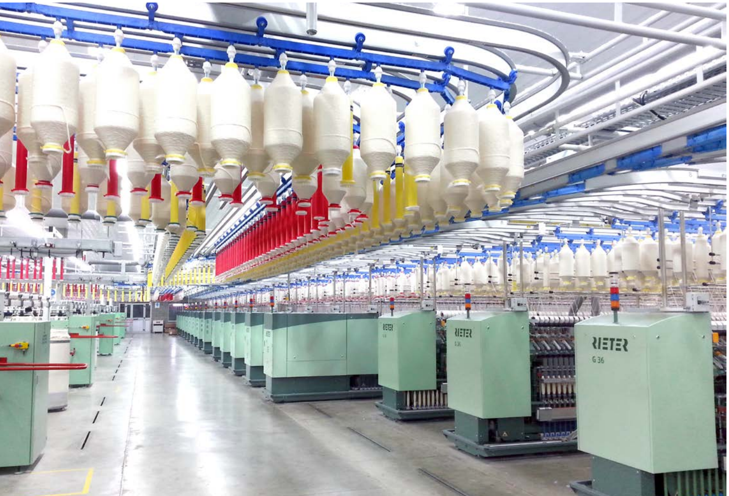
Fig. 3 Perfect, contact-free bobbin transport ensures consistent quality.
